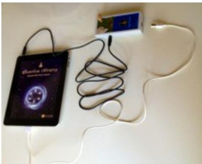
AFTER CONNECTING APPLE DEVICE CHARGER (# 4), CONNECT USB END TO THE IMPRINTER
